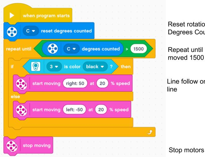
Reset rotation sensor (Reset Degrees Counted) on Motor C
